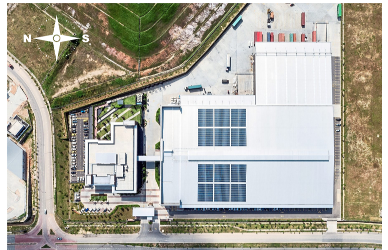
The building's long sides, where the warehouse and entrance are, face the morning and afternoon sun.
