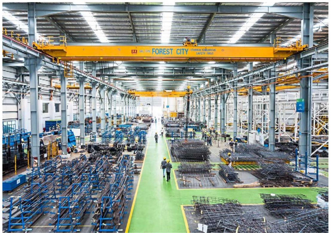
ABOVE Transparent roofs at Forest City industrialised building system plant provides natural lighting.
